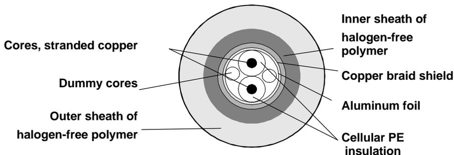
Figure 4-12 Structure of the SIENOPYR-FR Marine Cable
