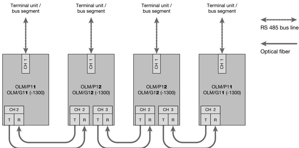
Fig. 2: Network structure in an optical line topology
