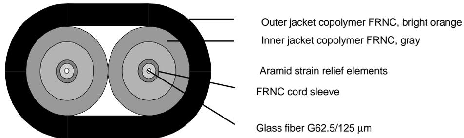
Figure 7-5 Structure of the INDOOR Fiber-Optic Cable
