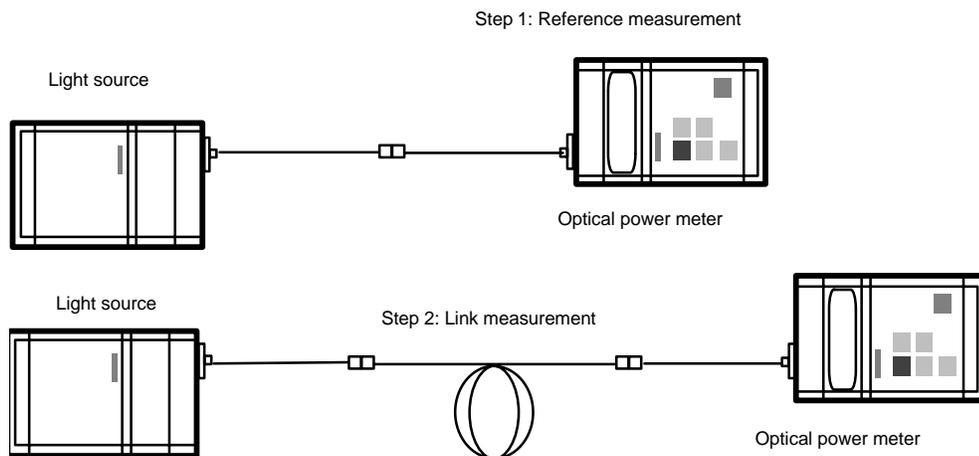
Figure A-2 Measuring the Total Attenuation of a FO Link
