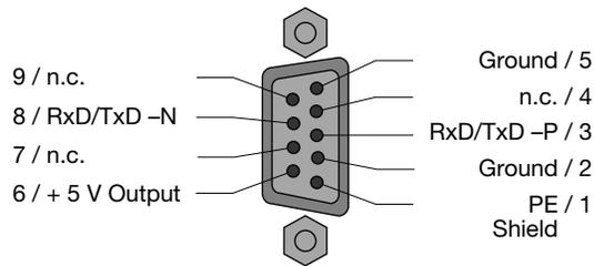
Fig. 9: Electrical port – assignment of Sub-D sockets
