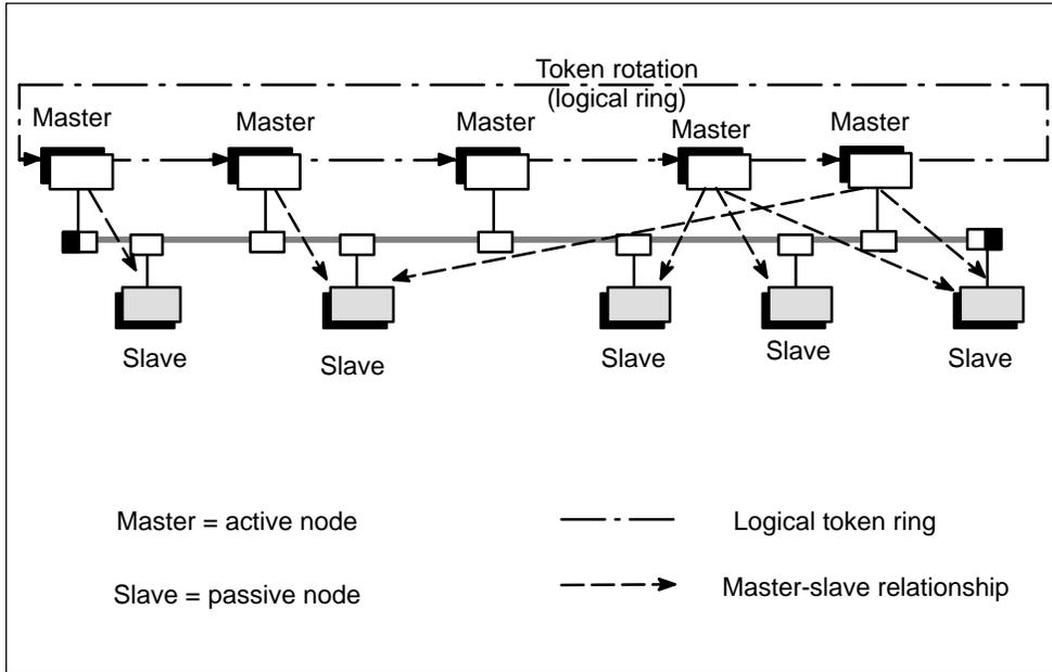
Figure 1-1 Principle of the PROFIBUS Medium Access Technique
