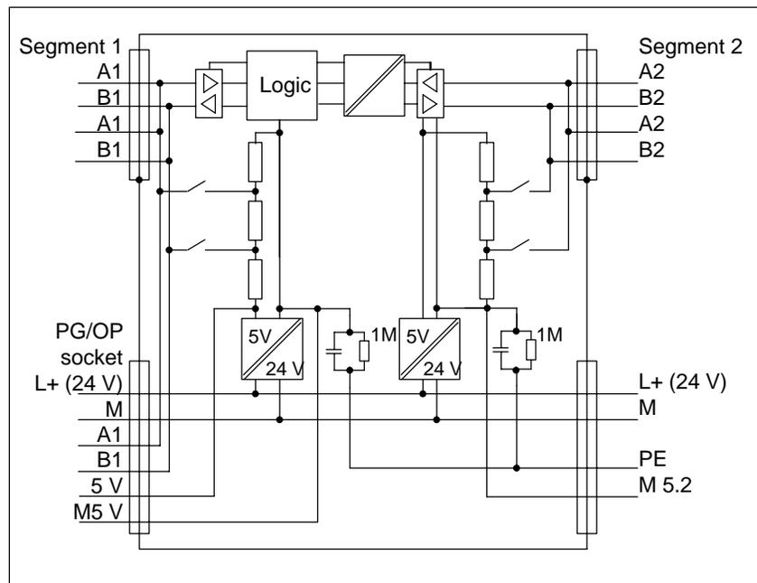
Figure 5-1 Block Diagram of the RS-485 Repeater
