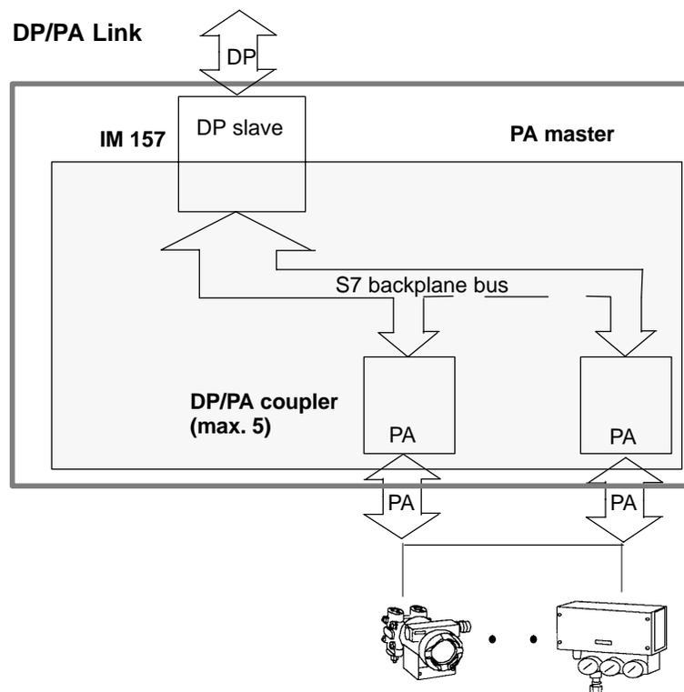
Figure 2-17 The DP/PA Link with DP/PA Couplers
