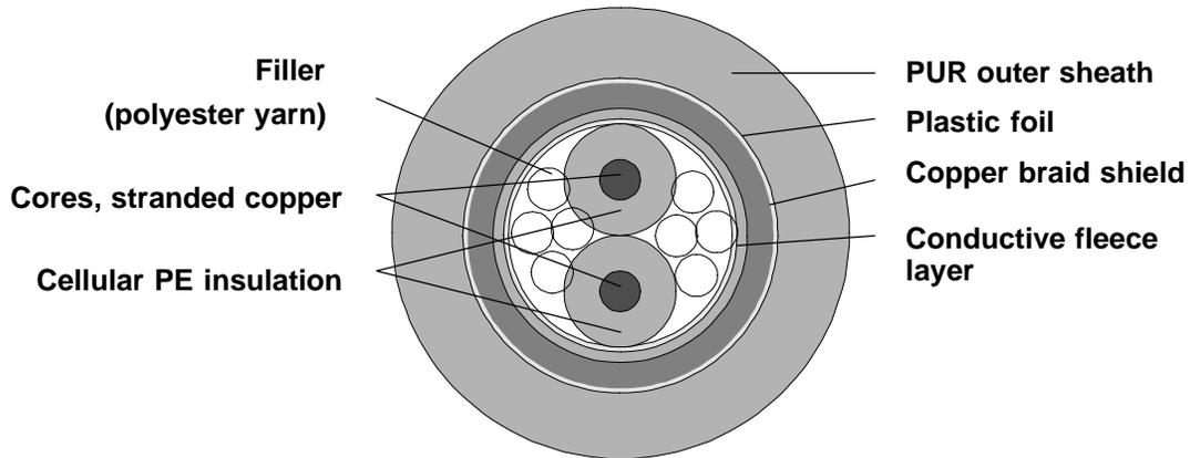
Figure 4-5 Structure of the Flexible Cable (Robot Cable)
