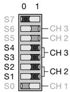
CH3 is activated in this operating mode if S3 and S4 are in Position 1.
