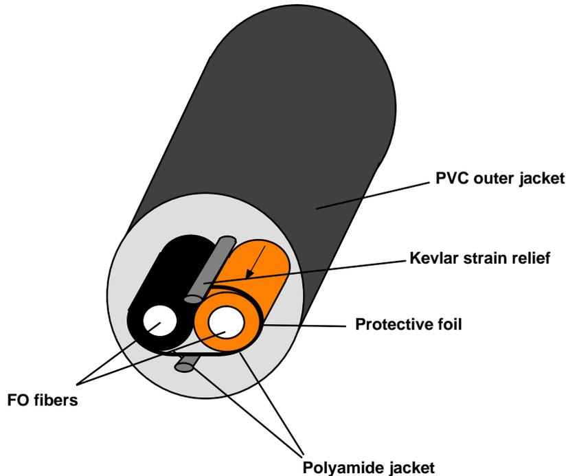
Figure 7-2 Structure of the Plastic Fiber-Optic Standard Cable
