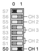
CH1 is activated in this operating mode if S0 is in Position 1.
