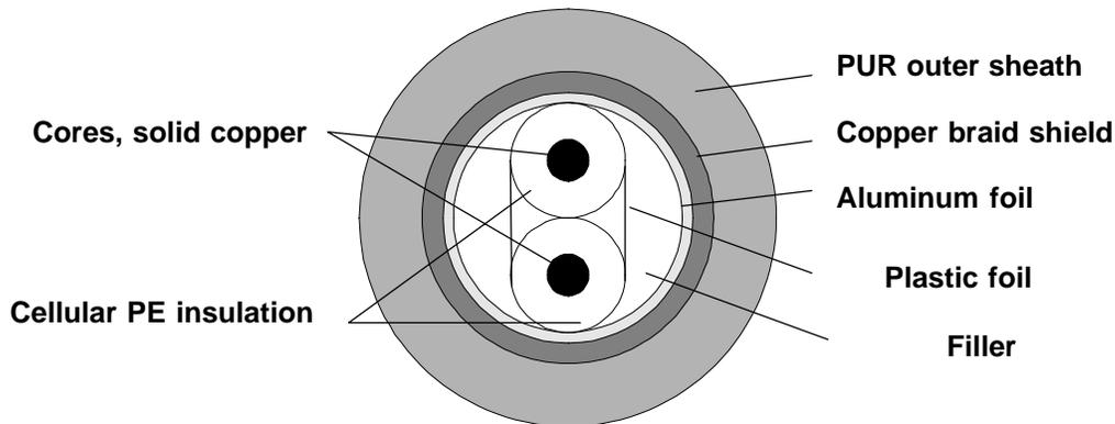
Figure 4-4 Structure of the FC Robust Cable
