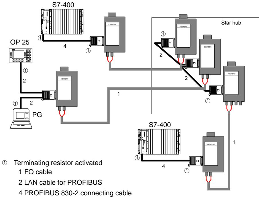
Figure 2-4 Example of a Star Topology with OLMs
