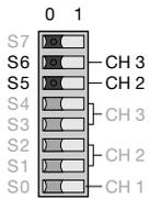
Switch S6 to Position 0 (reduced) if overloading is detected at a non-OLM device when using plastic optical fiber cables to CH3.
