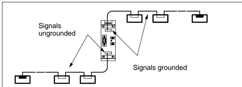
Figure 5-8 Ungrounded Operation of Bus Segments
