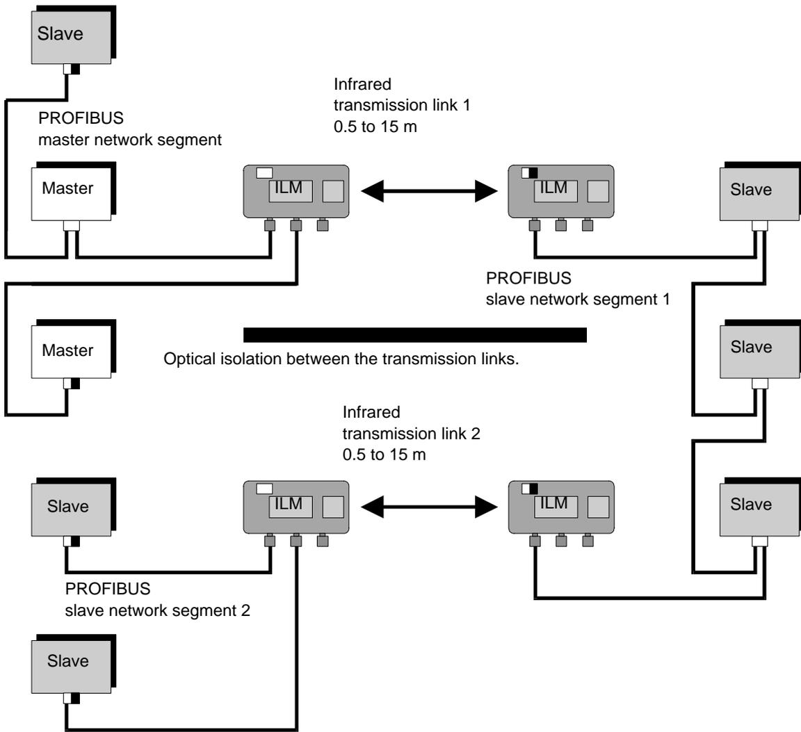
Figure 3: Cascading Two PROFIBUS ILM Transmission Links
