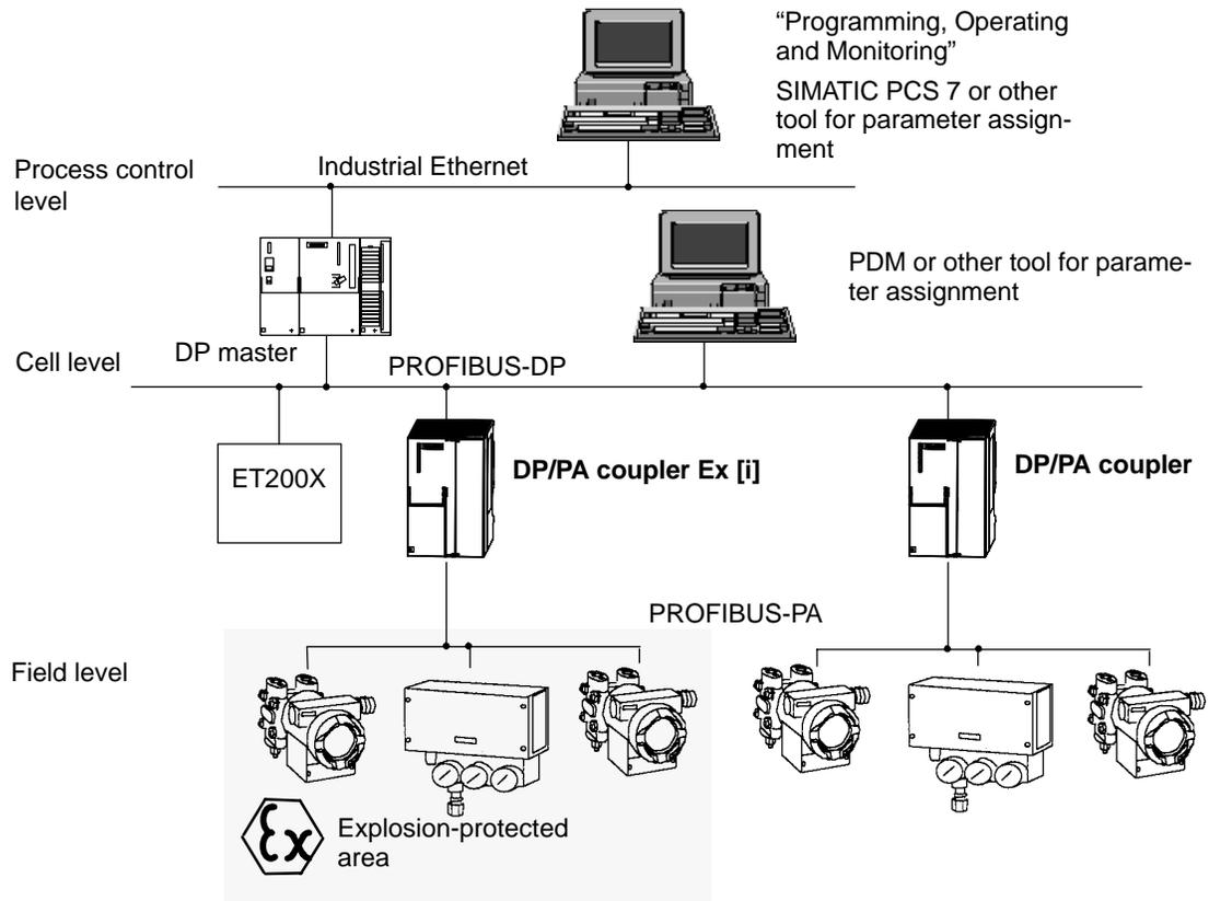
Figure 2-15 Linking the DP/PA Coupler into the System
