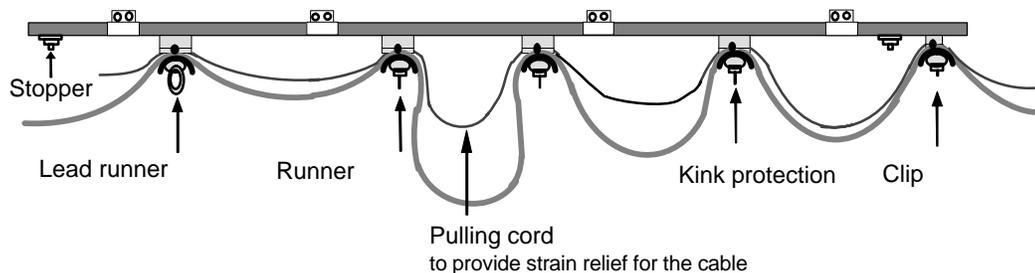
Figure 4-10 Installation of the PROFIBUS Festoon Cable (Schematic)
