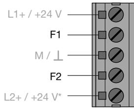
Fig. 12: Signaling contact – pin assignment 5-pin terminal block
