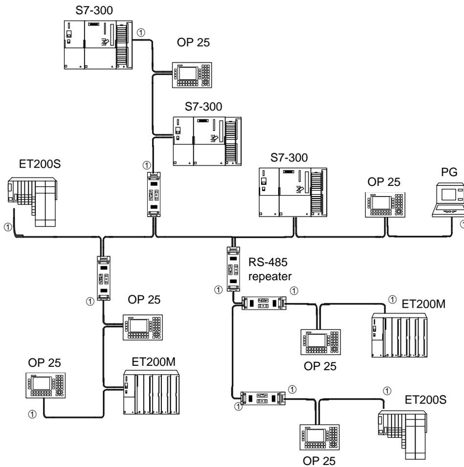
① Terminating resistor activated
