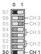
CH1 is activated in this operating mode if S0 is in Position 0.
