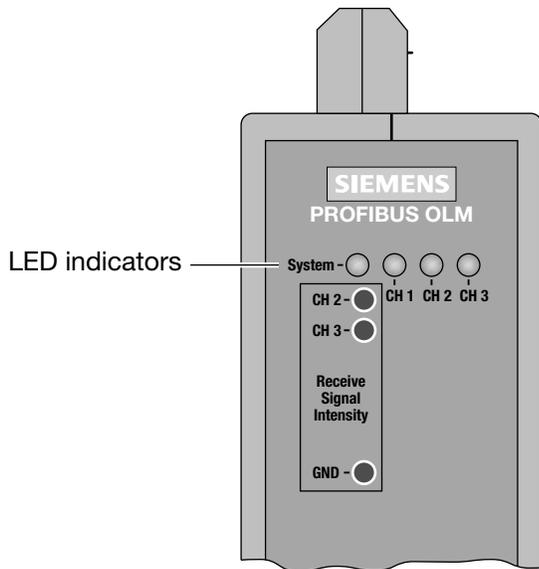
Fig. 14: LED indicators on the front plate
