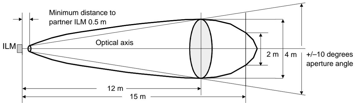
Figure 19: Transmitter Illumination of the PROFIBUS ILM
