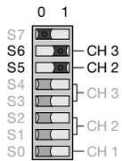
Leave S6 in Position 1 (default) if the optical fiber link to CH3 functions correctly in this position.
