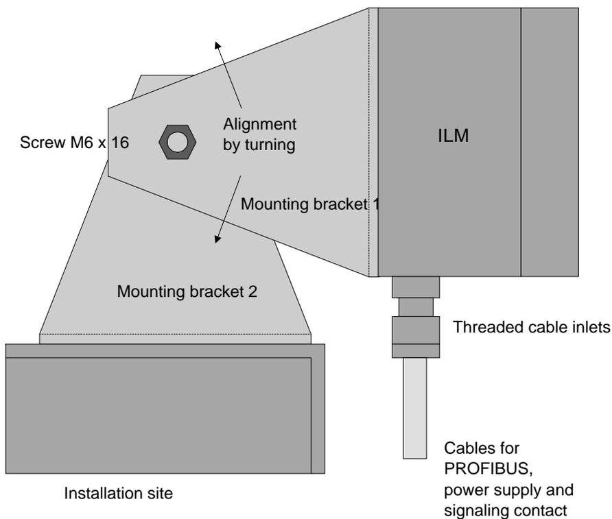
Installing the ILM with mounting bracket
