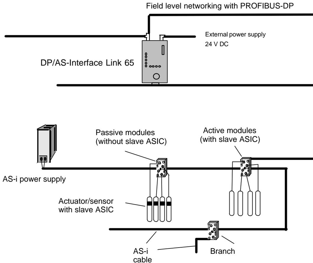
Figure 2-21 Example of a Configuration with DP/AS-Interface Link 65
