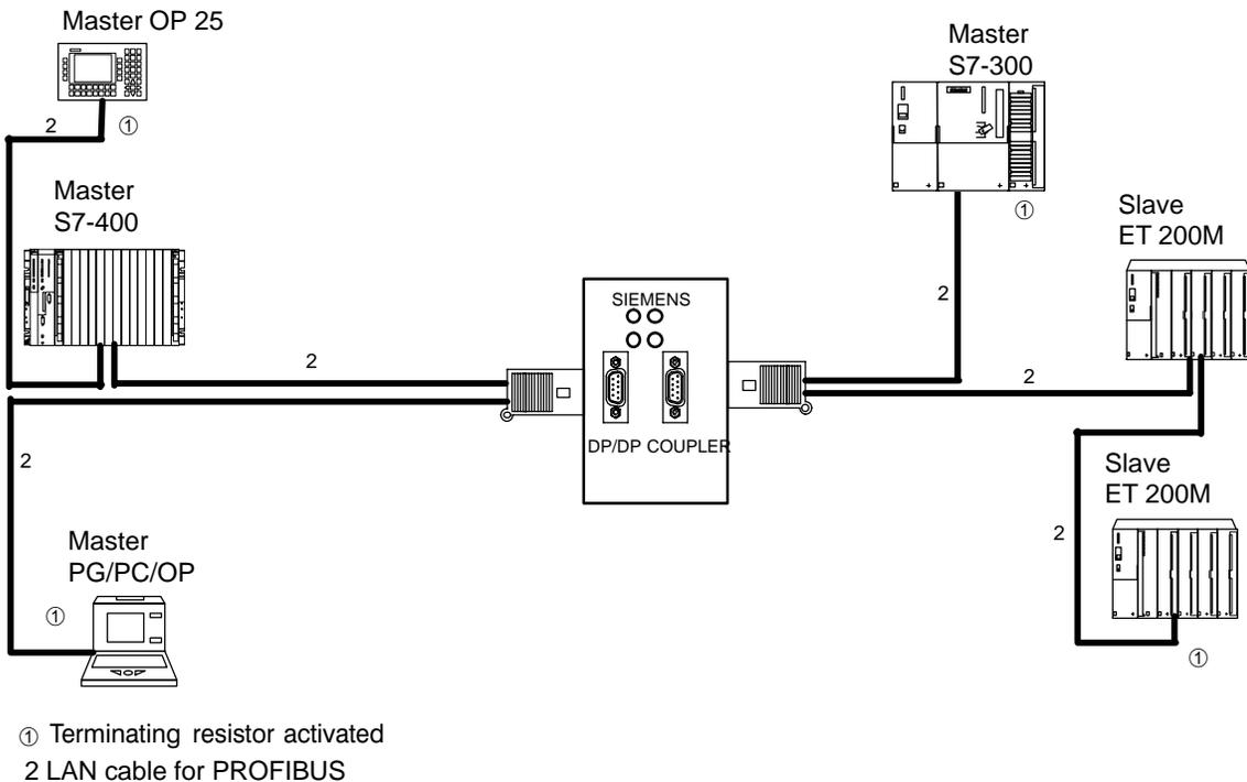
Figure 2-14 Configuration Example of the DP/DP Coupler
