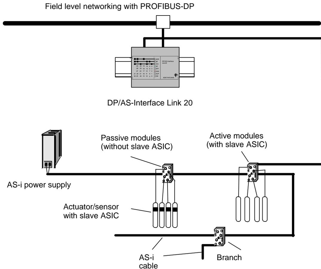
Figure 2-23 Example of a Configuration with DP/AS-Interface Link 20
