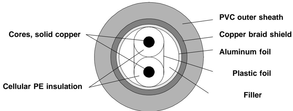
Figure 4-1 Structure of the FC Standard Cable
