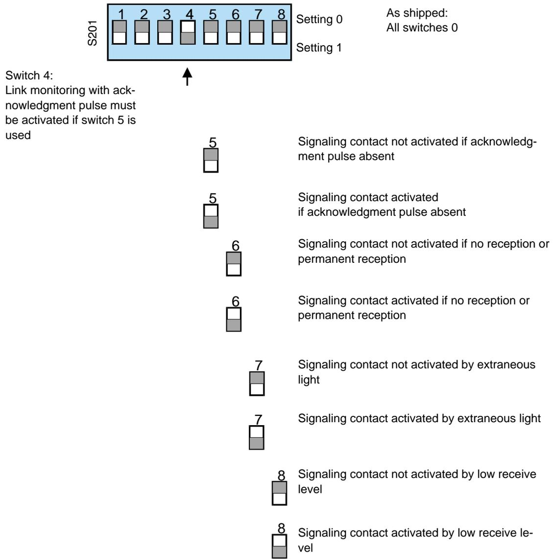
Figure 10: Configuration for Triggering the Signaling Contact
