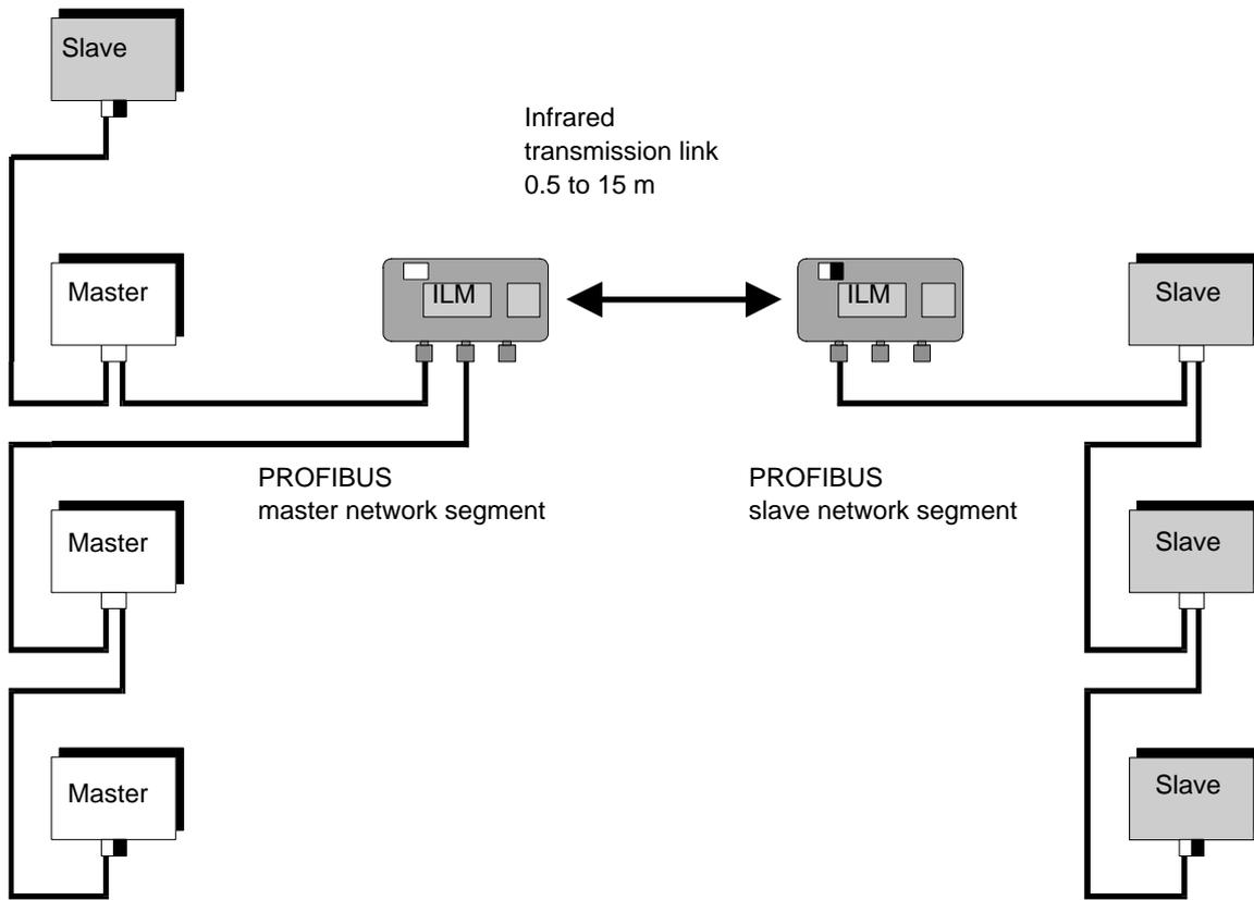
Figure 2: Point-to-Point Link with Two PROFIBUS ILMs
