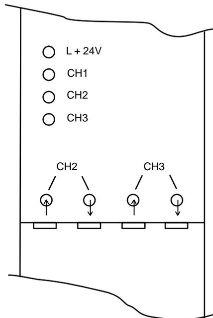
Figure 3-1 LED Displays on the Front Panel
