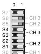
CH3 is activated in this operating mode if S3 and S4 are in Position 0.
