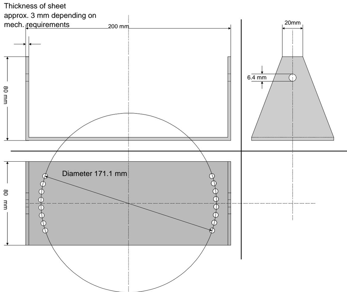
Figure 12: Example of a Simple Mounting Bracket
