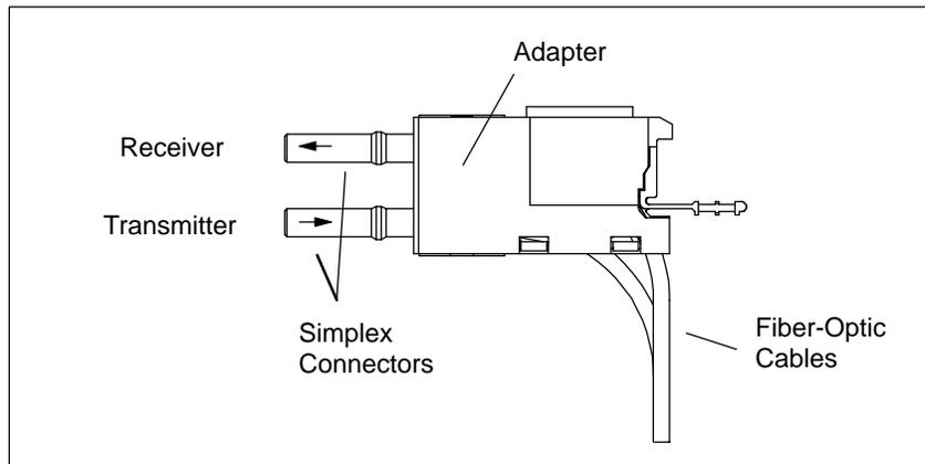
Figure 7-9 Simplex Connector and Special Adapter Fitted Together
