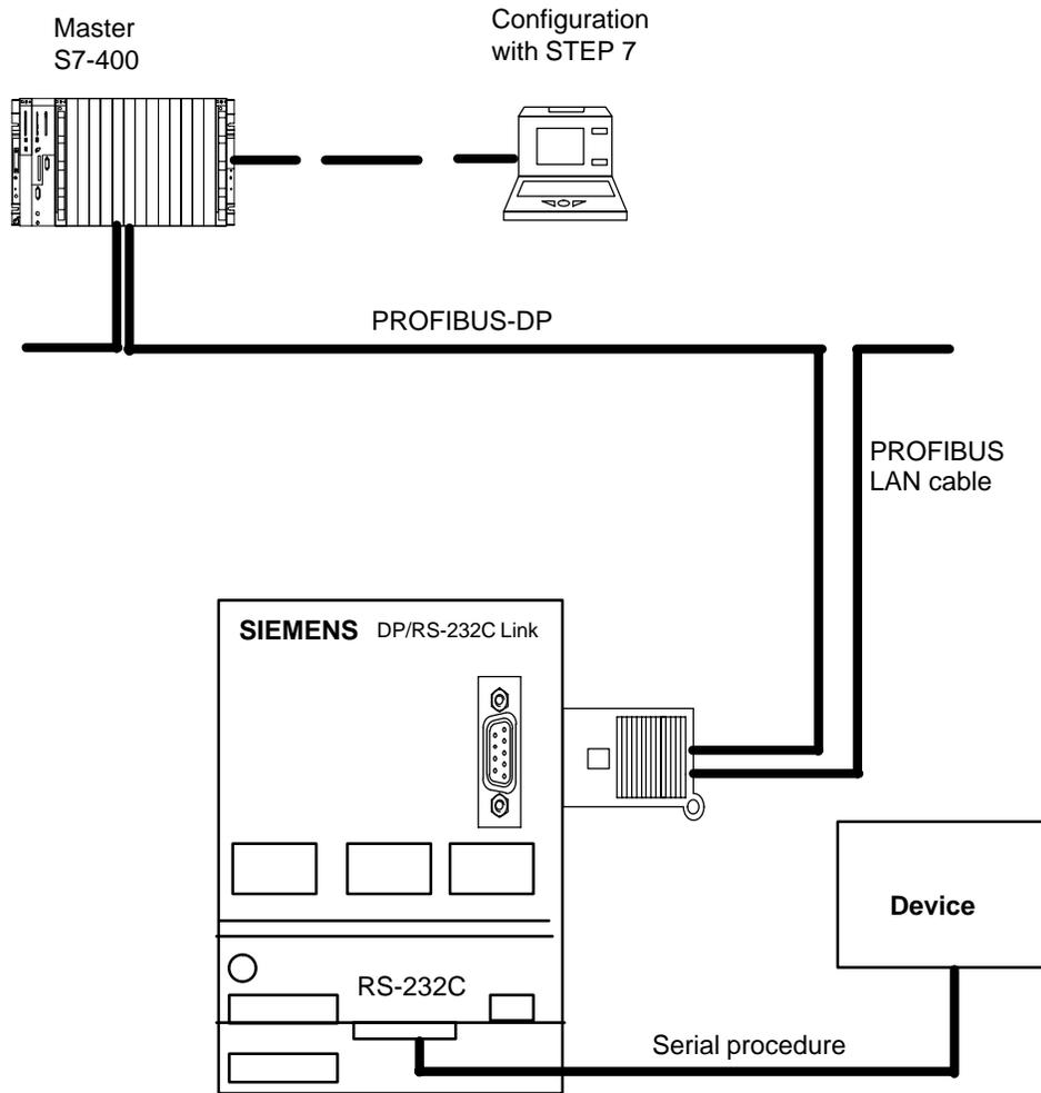
Figure 2-19 Example of a Configuration with DP/RS-232C Link
