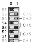
CH3 is activated in this operating mode if S3 is in Position 1 and S4 is in Position 0.
