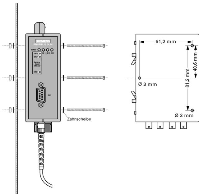
Figure F-18 Mounting the Optical Link Module OLM on a Mounting Plate
