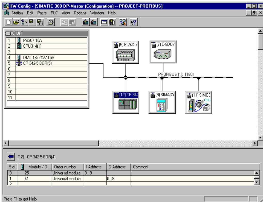
Figure 3-3 “HW Config” Dialog in STEP 7 (V5.0)
