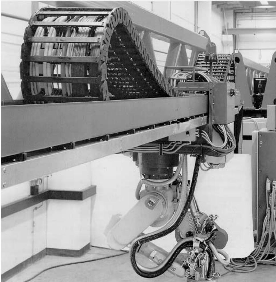
Figure 4-8 Example of Using the PROFIBUS Trailing Cable in a Drag Chain
