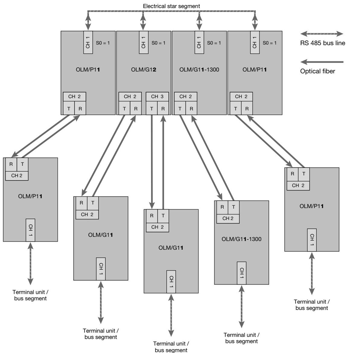
Fig. 3: Network structure in an optic star topology
