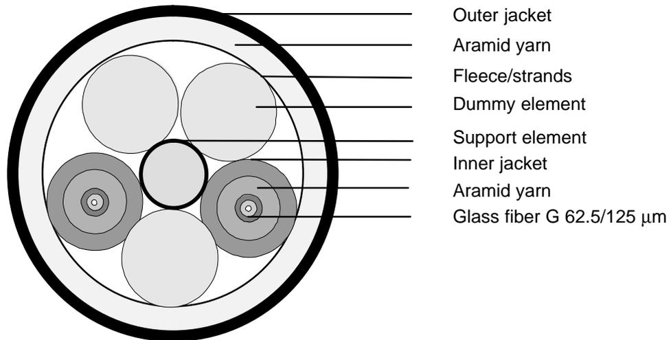
Figure 7-6 Structure of the Flexible Fiber-Optic Trailing Cable
