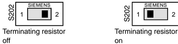
Figure 7: Setting the Terminating Resistor
