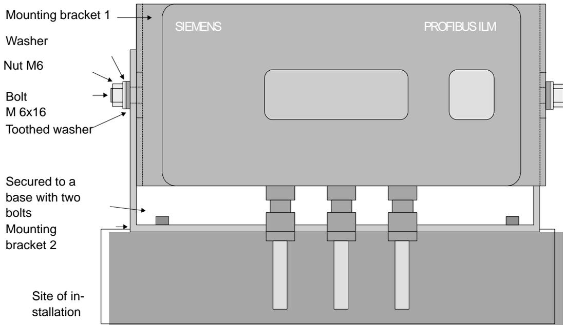
Installation of the ILM with a mounting bracket
