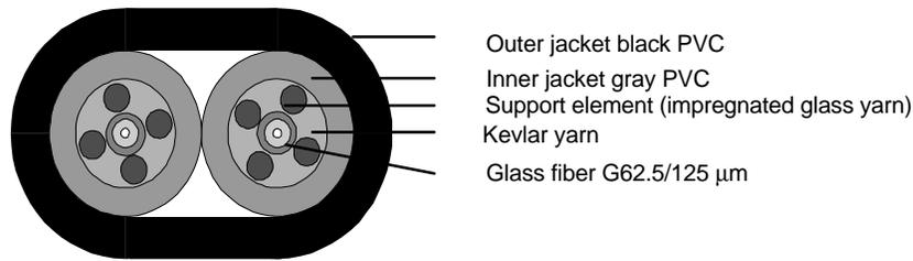
Figure 7-4 Structure of the Fiber-Optic Standard Cable
