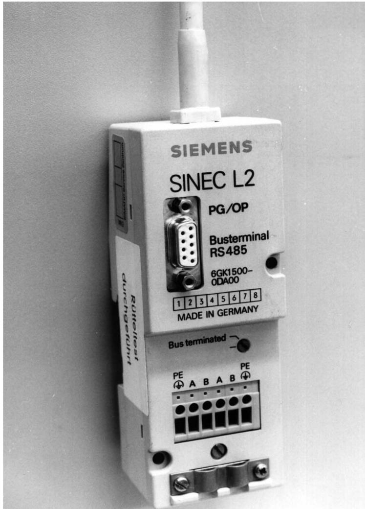
Figure 4-28 RS-485 Bus Terminal with Additional PG Interface
