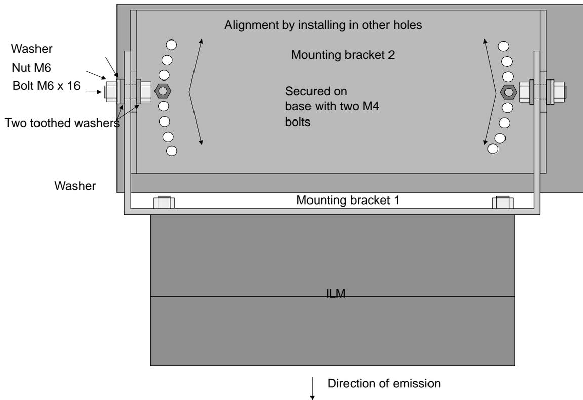
Installation of the ILM with mounting bracket
