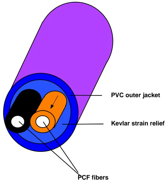
Figure 7-3 Structure of the PCF FO Standard Cable
