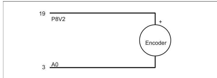
Figure 4-3 Connecting a NAMUR Encoder to Channel 0
