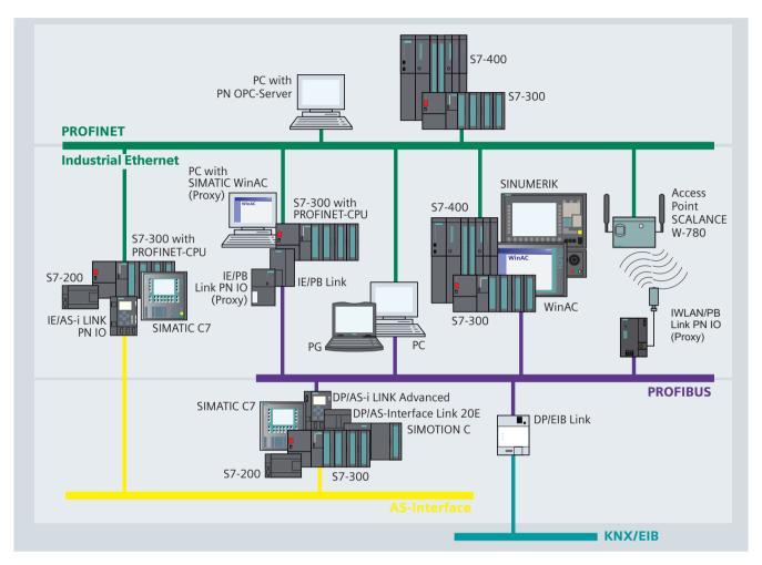
Network transitions between different bus systems are implemented through links, PLCs or PCs. In the latter 2 cases integrated interfaces and communications processors (CPs) are used. Links forward the data without any kind of changes from one network to another.
