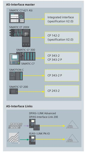
The DP/AS-i LINK Advanced or the DP/AS-Interface Link 20E (IP20) are available for connecting the AS-Interface directly to PROFIBUS DP, making it possible to use AS-Interface as a PROFIBUS DP sub-network.
