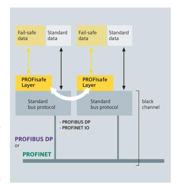
Using slave nodes, fail-safe encoder signals from a PROFIBUS station are transmitted to the fail-safe CPU. When these encoder signals have been logically linked an appropriate output signal is transmitted to a fail-safe PROFIBUS slave. Single channel transmission is used and there is no redundancy transmission path.
