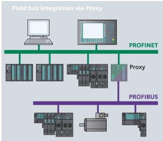
By integrating switch functionality into the devices, as is the case with the S7-300 with CP 343-1 Lean or the distributed field devices SIMATIC ET 200S or ET 200pro, the usual line structures can be formed which are directly adapted to the machine or plant structure. This makes cabling less complex and eliminates the need for components such as external switches.
