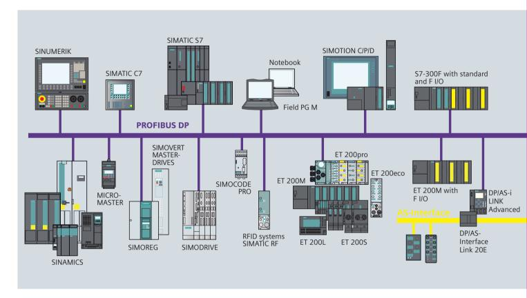
PROFIBUS is used for the connection of field devices such as distributed peripheries or drives with automation systems such as SIMATIC S7, SIMOTION, SINUMERIK or PCs.
