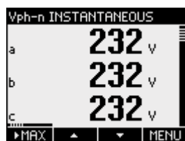
Figure 3-1 Display of the measured voltage in the case of connection type 3P4W
